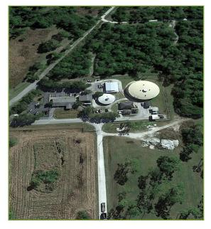
Our water treatment process consists of a series of steps. First, raw water is drawn from our water source and sent to an aerator, which allows for oxidation of the hydrogen sulfide and iron levels that are present in the water. Chloramines (chlorine and ammonia) are then added for disinfection. The water then goes into a ground storage tank from which sediment is removed.
